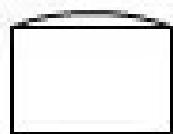
Dome Roof Tank
